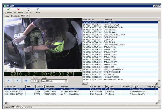
Since the data from both transactions and "events" (i.e., individual treadle activations, toll collector keypresses, ETC tag reads, gate activations) are replayed synchronously, you can quickly search for anomalous transactions, play them forward and backward in slow motion or high speed and ultimately understand the "hidden details" that caused the anomaly or incident.
